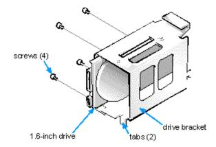
6. Align the four screw holes of the drive and bracket. Insert and tighten the screws that came with your upgrade kit (see Figure 11).
