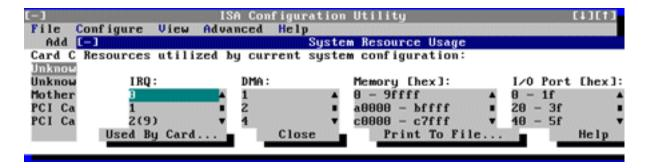
To determine which card uses a particular resource shown in the System Resource Usage dialog box, select the resource in question and then click Used By Card. The Card Resource Usage dialog box appears with the information.
