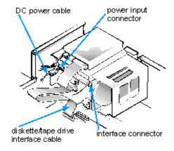
9. For an EIDE tape drive or CD-ROM drive, connect the other end of the interface cable to the interface connector labeled "IDE2" on the system board.
