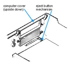
To replace the front-panel insert for the 3.5-inch bay, work from outside the cover. Place the insert in position, and press it into the opening.
