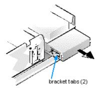
If a drive is already installed in the bay and you are replacing it, be sure to disconnect the DC power cable and interface cable from the back of the drive before sliding the bracket out of the bay. To remove the old drive from the bracket, turn the drive/bracket assembly upside down and unscrew the four screws that secure the drive to the bracket (see Figure 7).
