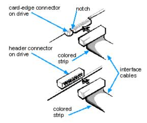
When attaching the interface cable to a drive, be sure to match the colored strip on the cable to pin 1 of the drive's interface connector. For the location of pin 1 on the drive's interface connector, see the documentation that came with the drive.
