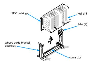
6. Insert the new SEC cartridge/heat sink assembly into the system board connector.
