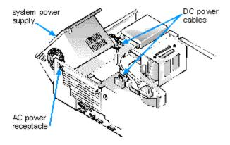
3. Free the power supply from the securing tab labeled "RELEASE —>, " and rotate it upward until it locks in its extended position.
