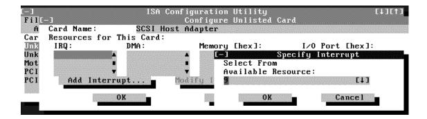
If you are providing a value for the IRQ or direct memory access (DMA) resource, click the down arrow beneath Available Resources. A smaller Specify list box appears (see Figure 8). Click the value you want to assign to the resource. Then click OK.
