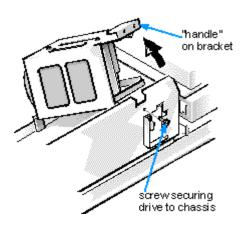
5. Slide the drive into the chosen bay of the bracket, orienting it so that the connector on the back of the drive will face the back of the chassis and the power input connector will be closest to the floor of the chassis when the bracket is reinstalled (see Figure 11).
