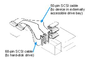
NOTICE: Do not connect devices to all three connectors (internal narrow connector, internal wide connector, and external connector) on a single SCSI host adapter card. Such a configuration is a violation of the SCSI specification. You can safely connect devices to any two of these three connectors on a single SCSI host adapter card.
