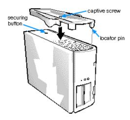
As you lower the stand into place, make sure that the locator pin (see Figure 4) fits into the corner hole of the hole pattern as shown. When the stand is in place, tighten the thumbscrew.
