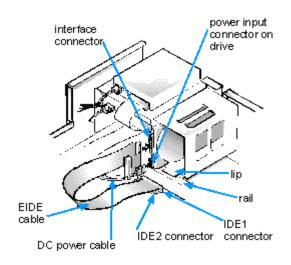
NOTICE: You must match the colored strip on the EIDE cable with pin 1 on the system board IDE connector to avoid possible damage to your system.
