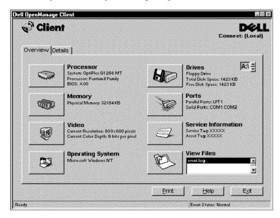
On systems running Windows 95, Windows 98, and Windows NT 4.0, the Dell OpenManage program is available in client and administrator versions. The Dell OpenManage administrator version enables system administrators to view, manage, and inventory remote systems in a Dell DMI client network and incorporates the following manageability features, which are based on the DMI 2.0 specification.
